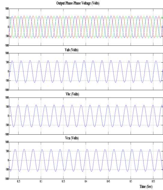
Fig. 15(a). Output voltage and current waveform during normal power supply.
