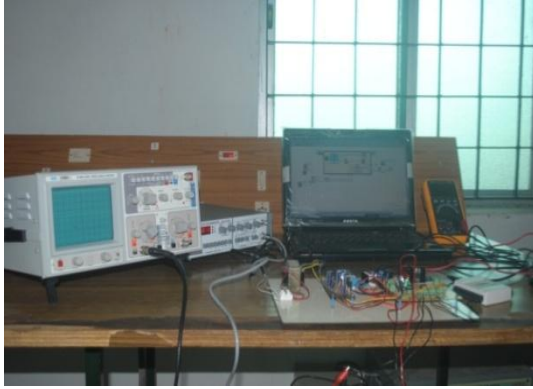
Fig .6 (a) GPI controller Setup for Buck converter
