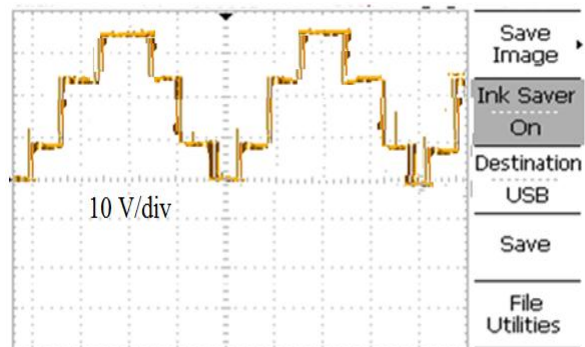
Fig. 10. Voltage level in switching devices for different switching time period
