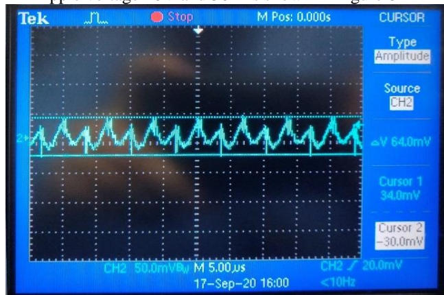
Figure 8: Ripple voltage at Vin-nom and Iout-max
