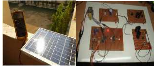
Fig. 20. Hardware implementation of semi ZSI with 1211-SUNSTAR solar Panel.
