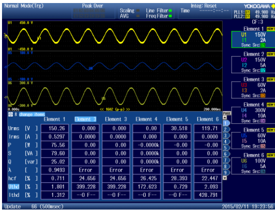
Fig.25. Experimental results for 25% voltage swell
