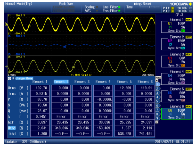
Fig 23. Experimental results for 11% voltage swell
