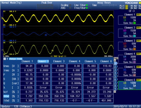
Fig 21. Experimental results for 21% voltage sag
