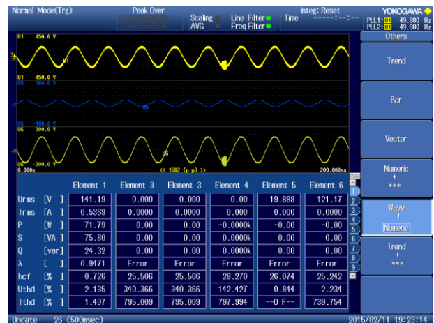
Fig 24. Experimental results for 18% voltage swell
