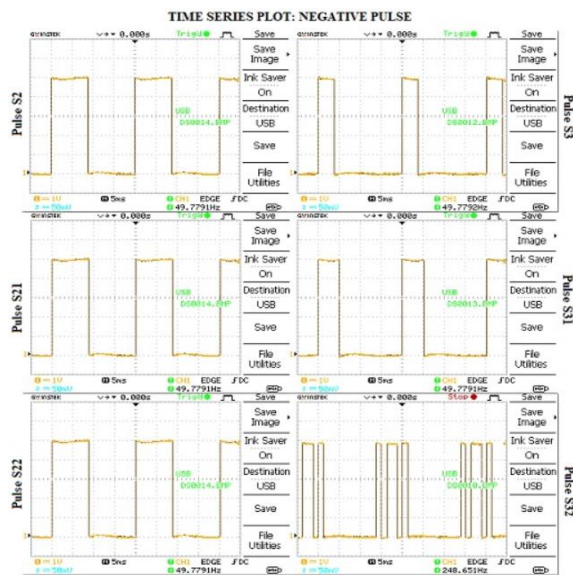
Fig. 3.2 a. Negative pulse pattern using PIC controller
