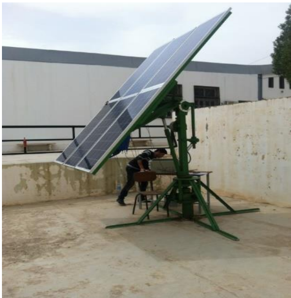
Fig. 2. Back view of the generator showing the effort multiplier and the hydraulic jack
