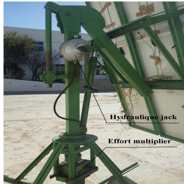
Fig. 2. Back view of the generator showing the effort multiplier and the hydraulic jack
