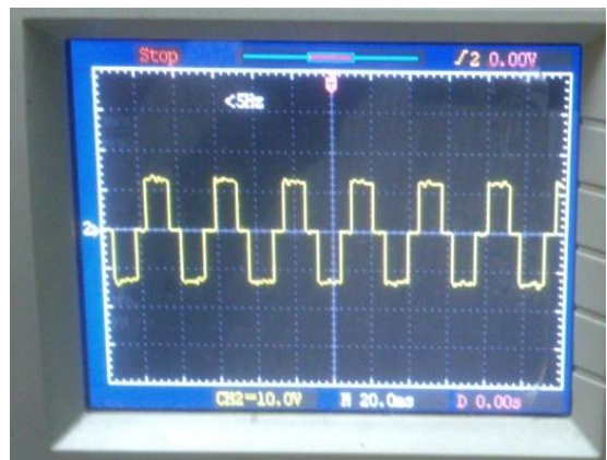
Figure.18. Line to Line Voltage
