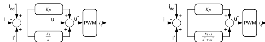
Fig. 9. Stationary PI (left) and stationary PR (right) current control for single-phase voltage source grid converters
