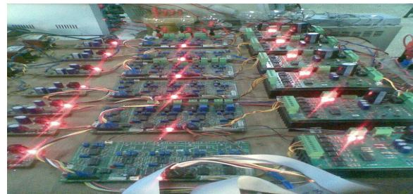
Fig.39. Hardware setup for three phase cascaded MLI
