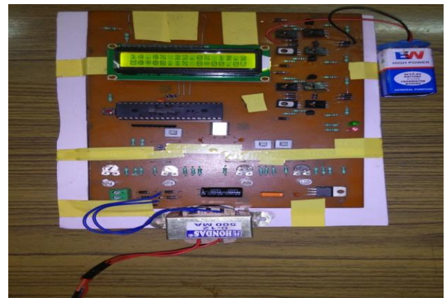
Fig.9. Hardware Components mounted (soldered) On the main Circuit Board
