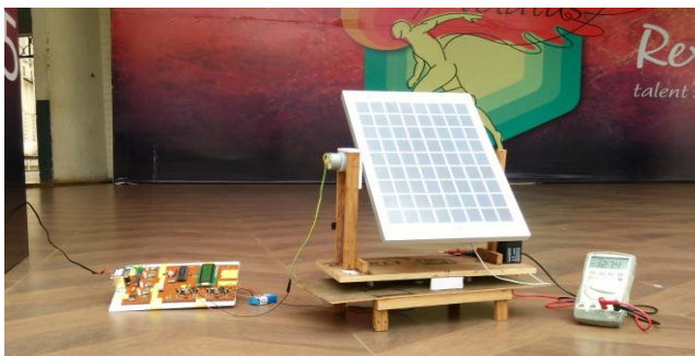
Fig.7. Dual axis Solar Tracker Testing
