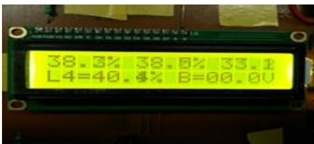
Fig.8. LCD status displaying the Light Intensities of different LDR Sensors
