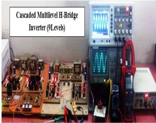
Fig.20. Experimental arrangement (b) CHBMLI (nine levels)
