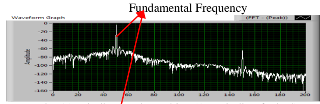
Fig. 11 Winding Fault machine (1% winding faulted)
