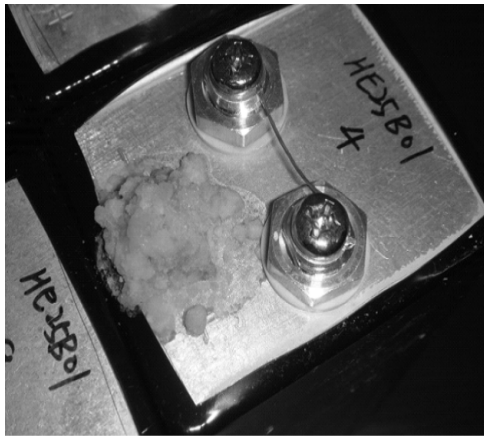
Fig.12. Showing the leakage of electrolyte during experimentation
