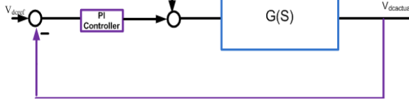
Fig. 3 Block diagram of an SMIB system with PI controller as a single input single output (SISO) system
