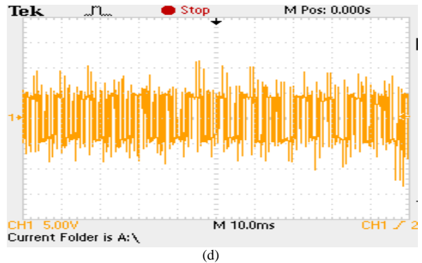
Fig. 6 Results of v/f controlled VSI fed induction motor drive with AZSPWM2 (a) Modulating signal, pulse pattern, Line Voltage and Line Current (b) Harmonic spectrum of Line Voltage (c) Harmonic spectrum of Line Current (d) Common Mode Voltage at M=0.86
