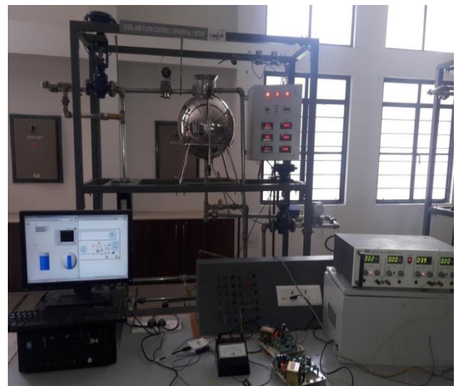
Fig. 6. Real time experimental setup of the Spherical Tank System
