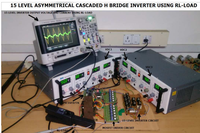
Fig. 34. 15-Level Asymmetrical CHBMLI with RL Load by using PIC16F877A
